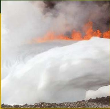
EXPANDOL Foam Concentrate is a blend of synthetic hydrocarbon foaming agents and stabilisers specifically selected to produce foams with a large expansion capacity and a high retention of water.
